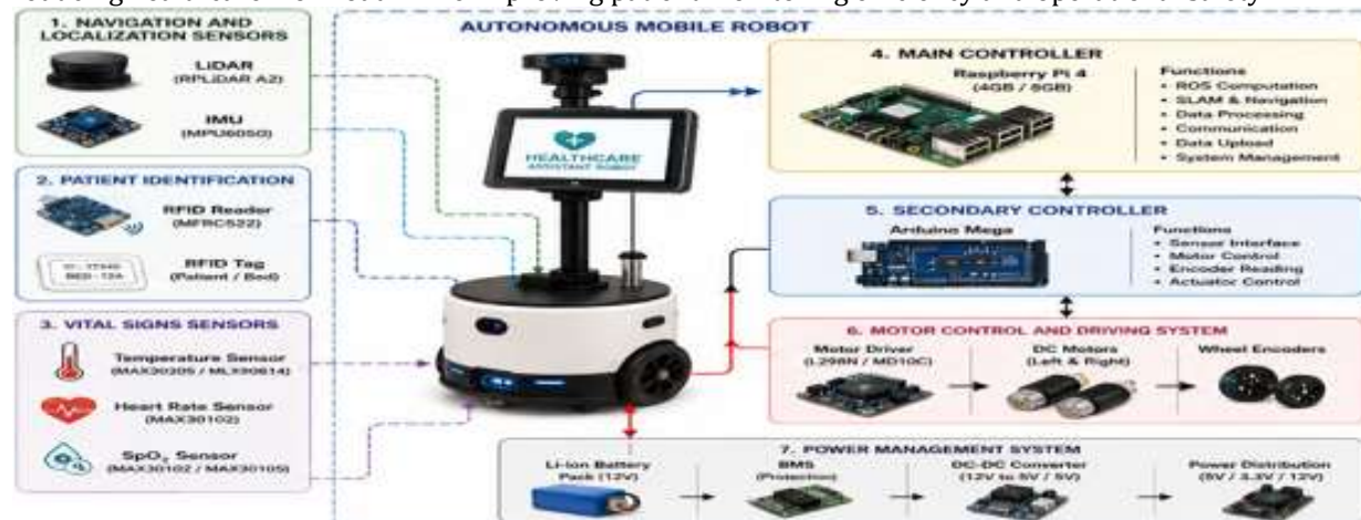
Fig. 1. Detailed architecture of the integrated autonomous mobile robot for vital signal surveillance
