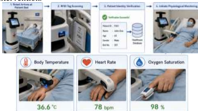
Figure 3. Autonomous Navigation, RFID Verification, and Vital Signs Acquisition Process
