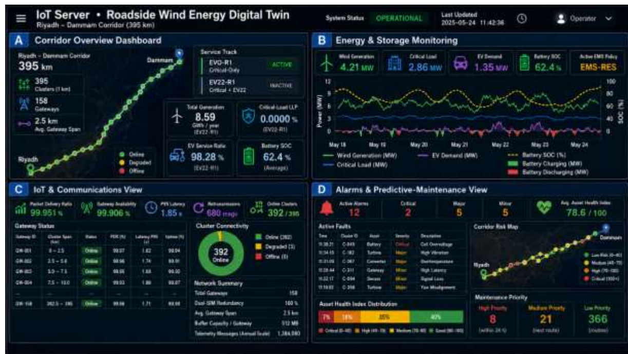
Figure 17. IoT server and data-visualization interface of the proposed roadside wind-energy digital twin: (A) corridor-level overview showing the 395 km Riyadh–Dammam corridor, cluster and gateway status, service-track configuration, generation, energy-based critical-load LLP , EV service , and battery SOC; (B) energy and storage monitoring showing wind generation, critical and EV demand, battery charging/discharging, SOC, and the active EMS policy; (C) IoT communication view showing gateway status, PDR, availability, P95 latency, retransmissions, and online/offline clusters; and (D) alarm and predictive-maintenance view showing active faults, severity, asset-health index, corridor location, risk class, and maintenance priority. LLP in the graphic denotes the energy-based critical-load index defined in Equation (22).
