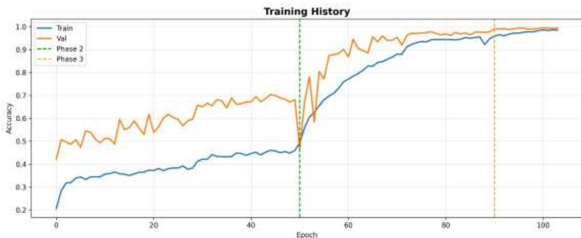
Figure 6: Training and validation accuracy across 105 epochs. Green dashed line = Phase 2 transition (≈epoch 50); yellow dashed line = Phase 3 transition (≈epoch 90). The brief dip at Phase 2 onset reflects cosine-annealing warm restarts.
