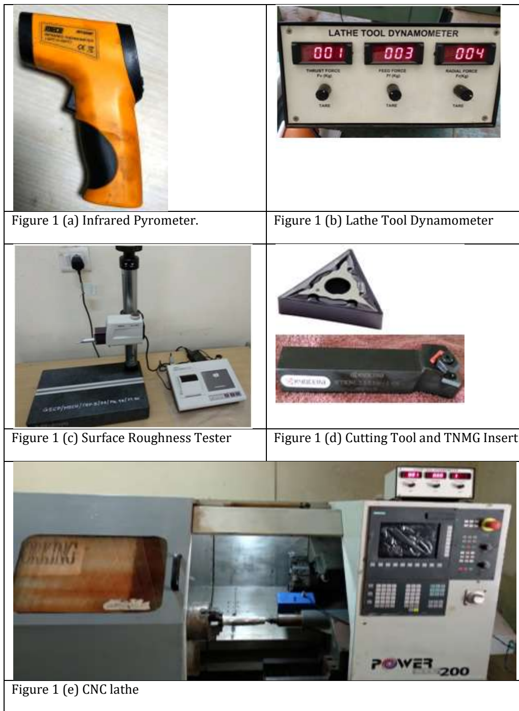
Figure 1 Machine and equipments used for experimentation
