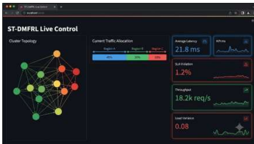
Figure 6.5. Real-time inference interface: live cluster topology, current traffic allocation and instantaneous latency, SLA and throughput indicators.
