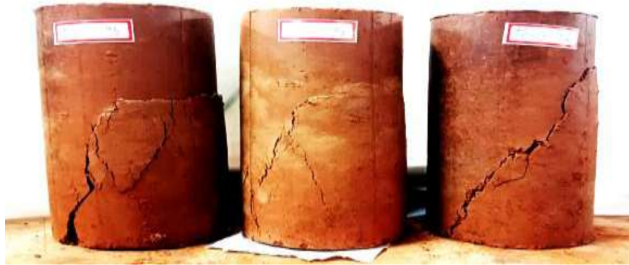
Fig. 9. Failure patterns of specimens reinforced at (A) H/2 , (B) H/3 , and (C) H/4 .
