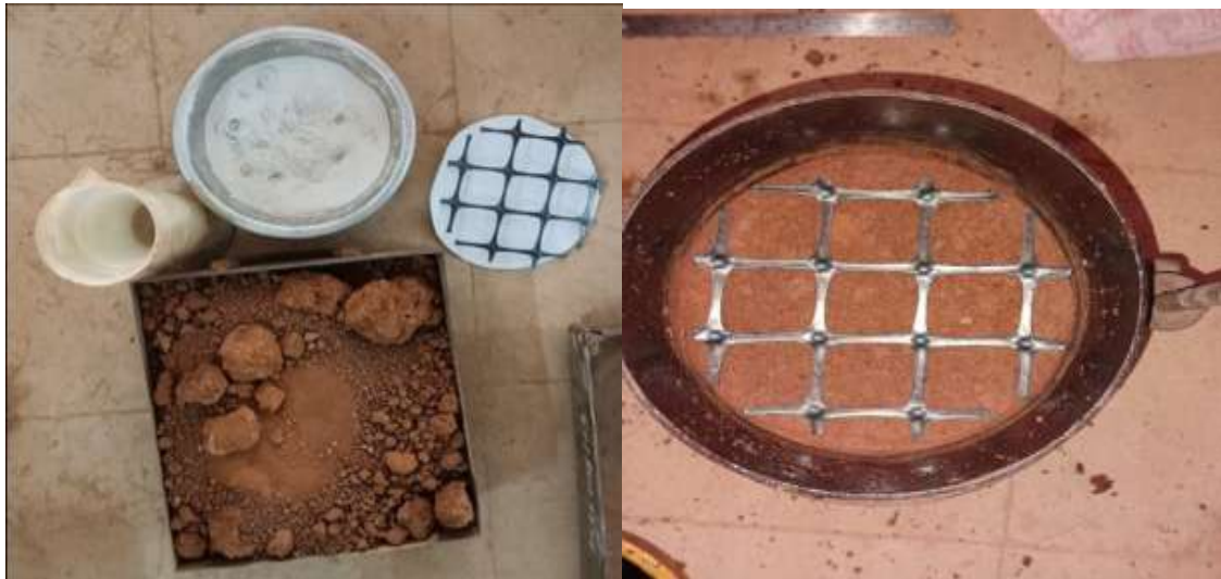
Fig. 2: Placing of geogrid at predetermined depth.
