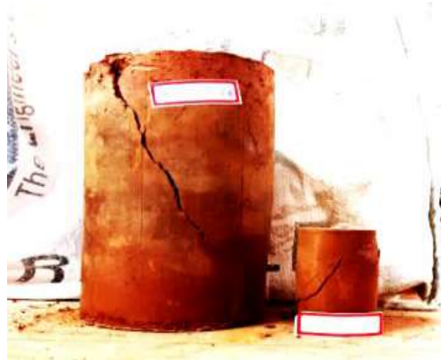
Fig 8: Failure patterns in large-scale (A) and small-scale (B) UCS specimens stabilized with 10% Fly Ash.
