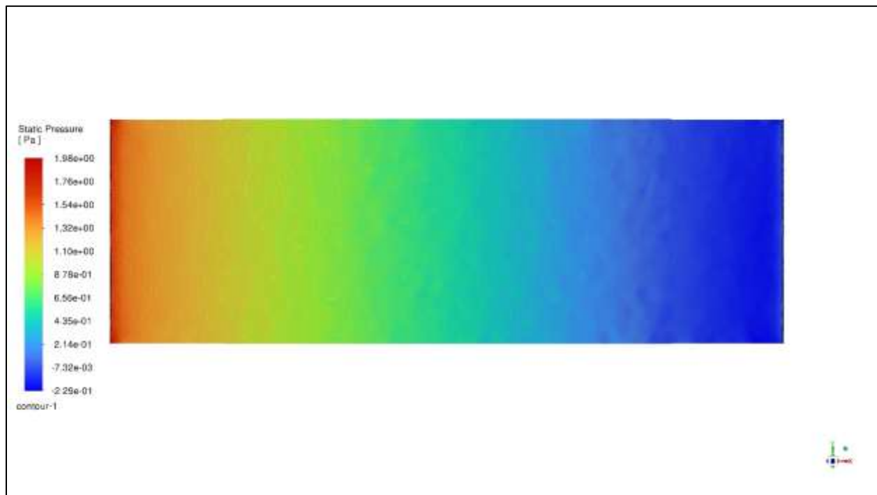
Figure 9 the static pressure contour for the smooth SAH duct
