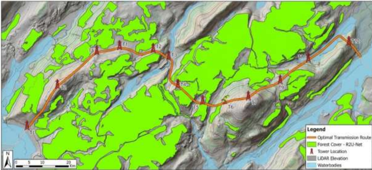
Figure 2: A high-resolution spatial map overlay of the final autonomous transmission corridor. The image highlights the route successfully winding between dense forest canopies, identified in bright green via R2U-Net segmentation, with precise tower locations spotted on optimal topographical gradients derived from the underlying LiDAR terrain model.
