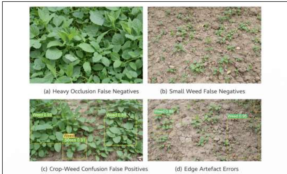
Figure 5. Analysis of Failure Cases: (a) False Negatives due to Heavy Occlusion, (b) Small-Weed Misses, (c) Crop-Weed Confusion, and (d) Edge-Artifact Errors
