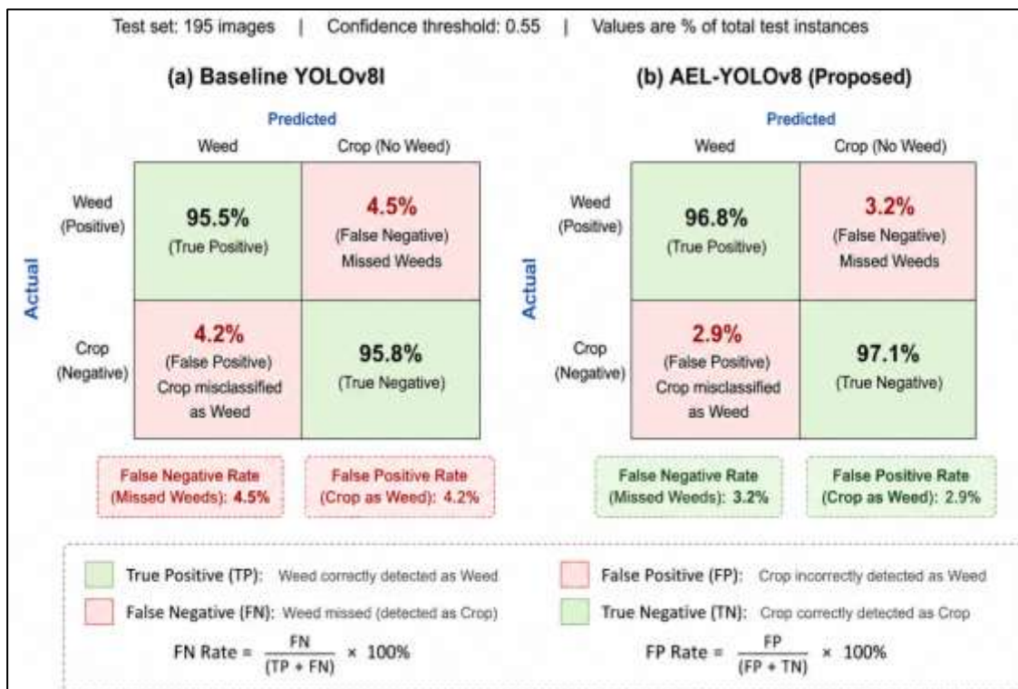
Figure 3. Confusion Matrices comparing AEL-YOLOv8 and the Baseline YOLOv8 on the Test Set
