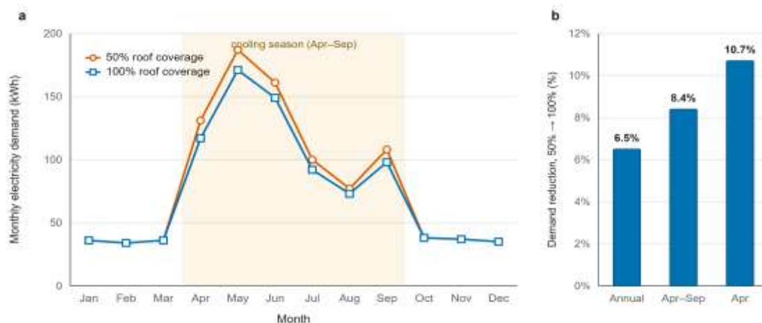
Fig. 3. (a) Archived monthly demand at 50% and 100% roof coverage; the shaded band marks the April to September cooling season. (b) Demand reduction from doubling coverage, over the year, over the cooling season and in the month of largest effect.
