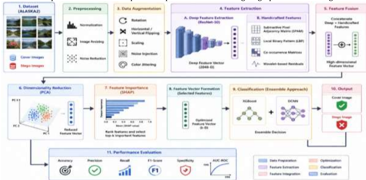
Figure 2: Proposed deep feature extraction and machine-learning-based steganalysis framework.
