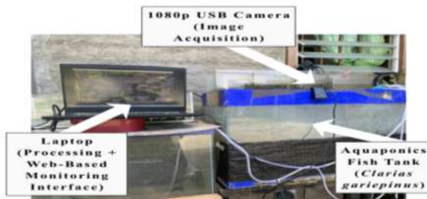
Fig. 3. Automated aquaculture monitoring system setup.
