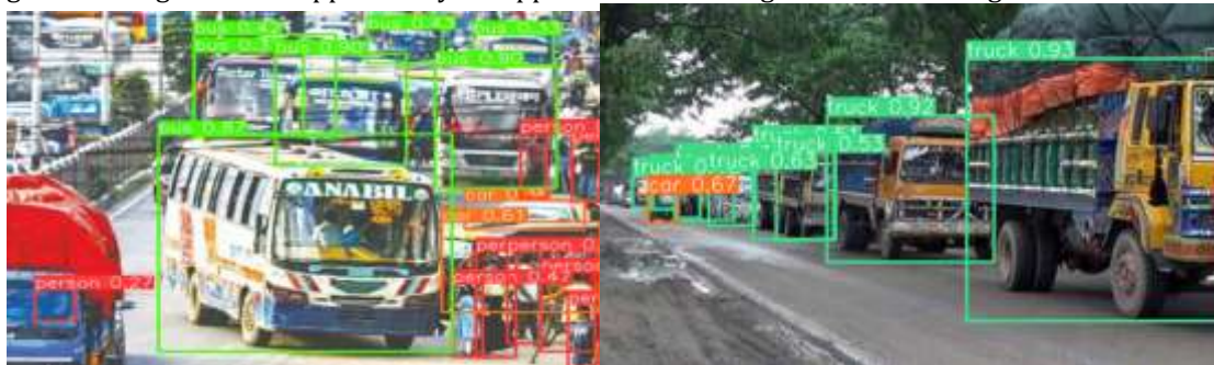
Figure 3: Detected images using YOLOv8 model.
