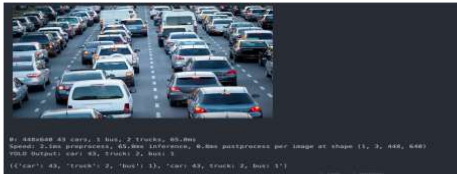
Figure 4: Detection of classes and text description result
