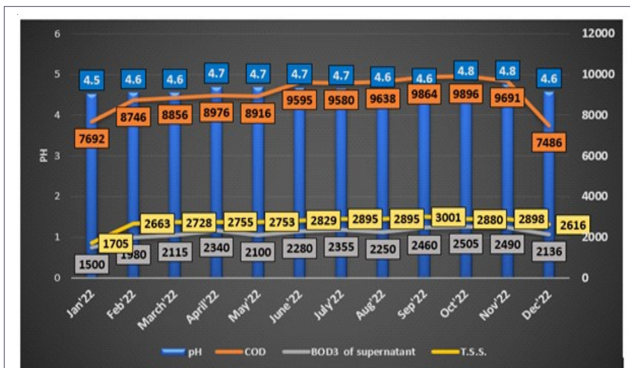
Figure 1: pH, COD, BOD and TSS Values of Composite Sample of Untreated Wastewater from Equalization Tank. All Values are in mg/l Except pH
