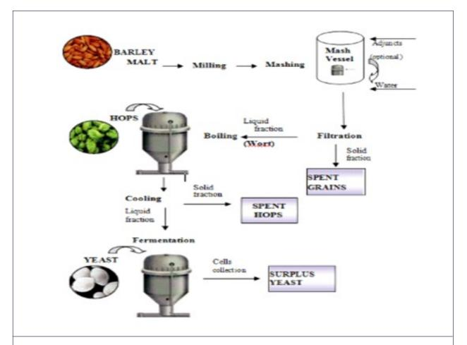
Figure 1: Schematic Representation of the Brewing Process and the Points Where the Main by-products are Generated
